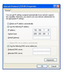
Figure 54: Internet Protocol (TCP/IP) Properties Window
